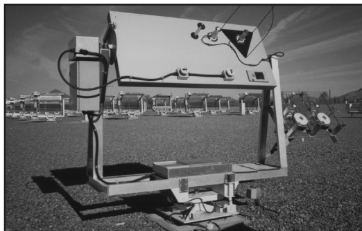
Figure 11. Radiant dosage calculations are made from data collected from a solar tracking device equipped with two Eppley TUVs and a Normal Incidence Pyrheliometer.
