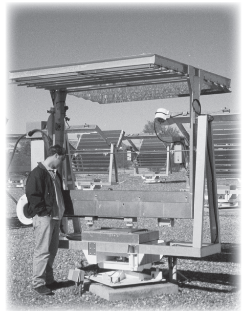
Figure 8. The 5 degree inverted lock-down position simulates dew formation on specimens during nighttime wetting. The lock-down position also allows easy specimen mounting and evaluation.
