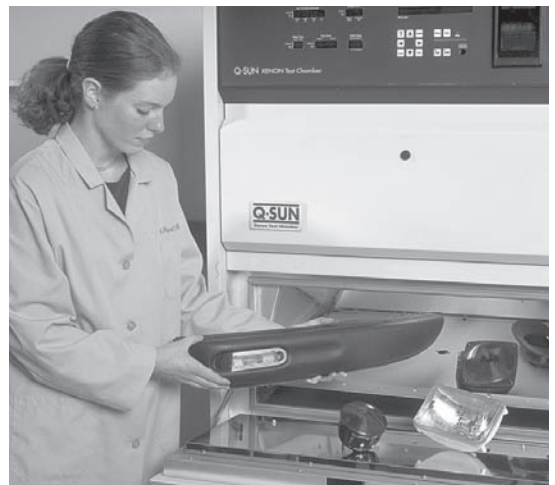
The Q-Sun Xe-3 accommodates 3-D parts, test tubes and petri dishes in addition to flat panels.
